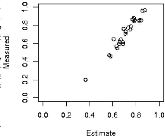
Examples of condition projection curves and historic condition measurement points are provided in the chart of figure 4. As an additional benefit of the approach, measurements off the condition projection line identify generators behaving inconsistently from their design and operation and so provide better outlier identification and direct further investigations.
