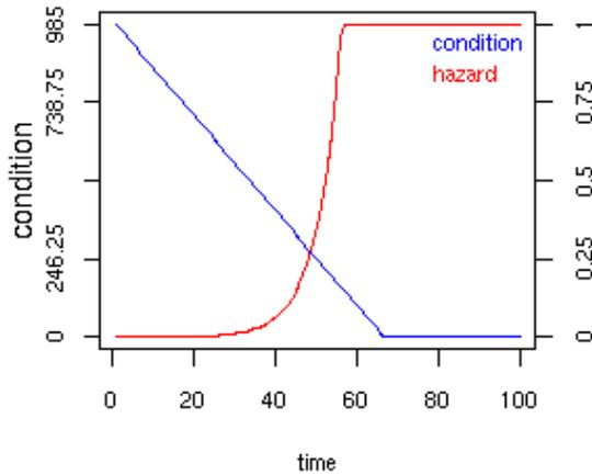
strength (viz condition) decreases and it becomes exposed to an increasing proportion of the distribution of external stress against which it will fail, as illustrated by the red shaded areas in the figure. These shaded areas represent the probability of physical failure with changing condition from which we can derive the hazard curve as illustrated in figure 6, that shows on separate axes the change in condition with time and the failure hazard with time.
