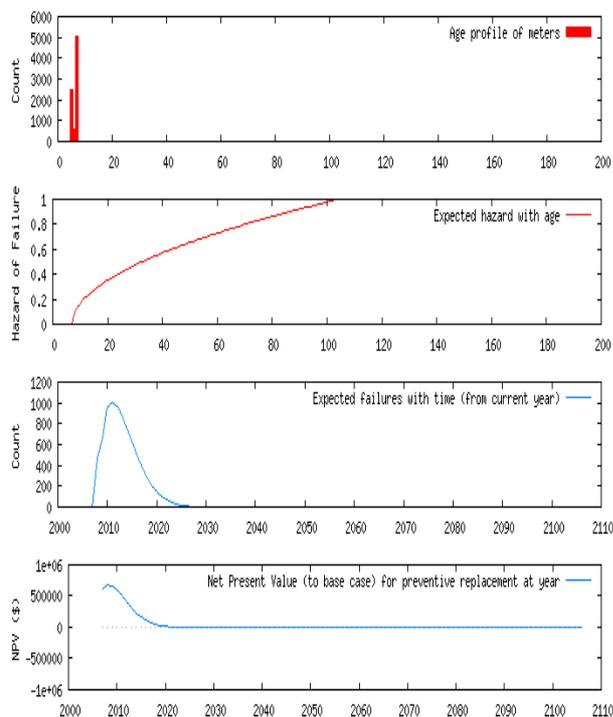
Figure 10: Meter Replacement Optimisation: Age Histogram; Failure Hazard with Age; Failure Numbers with Run-to-Failure; Relative NPV for Preventive Replacement
