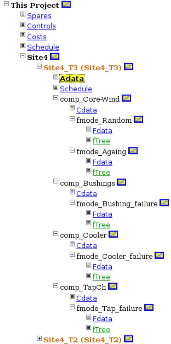
Figure 4: Transformer failure modes structure
