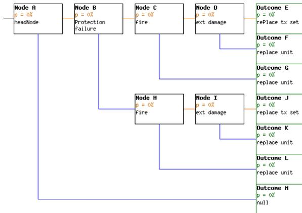
Figure 5: Core-winding failure consequence tree
