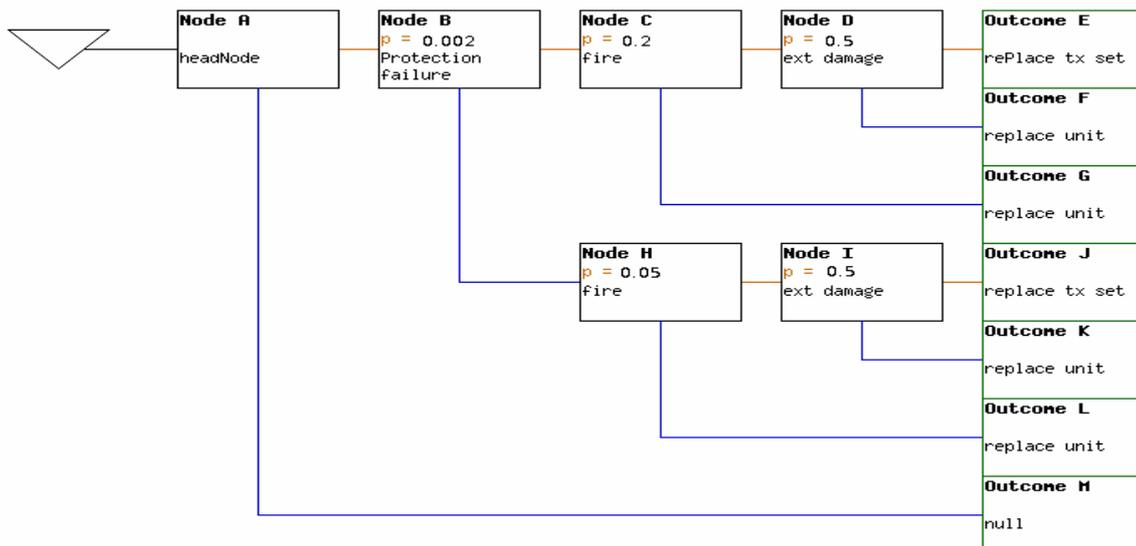
Figure 1. - representation of failure consequences.
